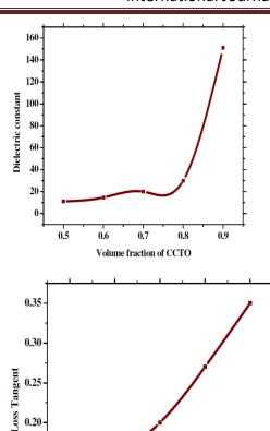
**Fig.1** Dependence of dielectric constant and loss tangent of the CCTO-silicone resin composites on the volume fraction of CCTO at 1 kHz and room temperature.
