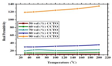
**Fig. 3** Dielectric constant vs. temperature for composites with different CCTO volume fraction at frequency 10<sup>3</sup> Hz.
